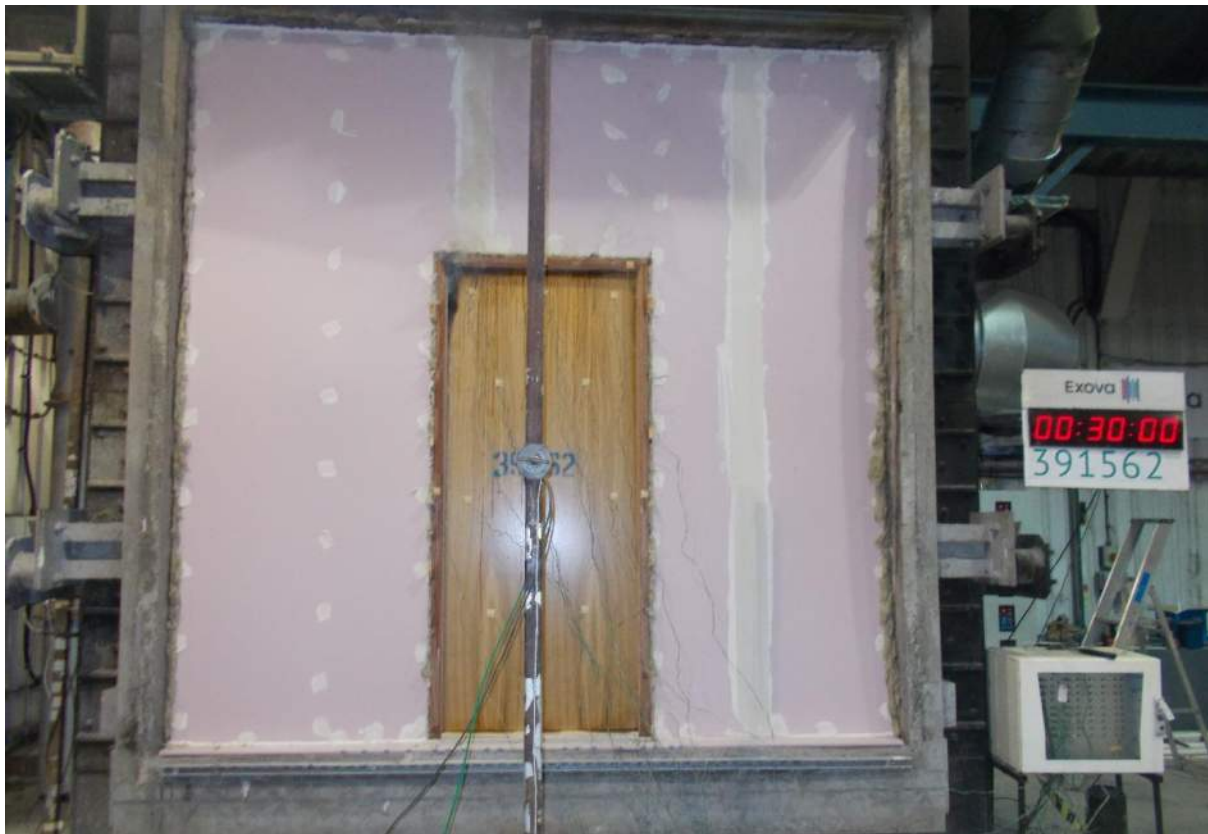
Exposed face – post test
